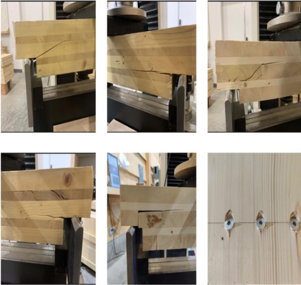
Figure 5: Different types of Shear Failures in 140mm series
