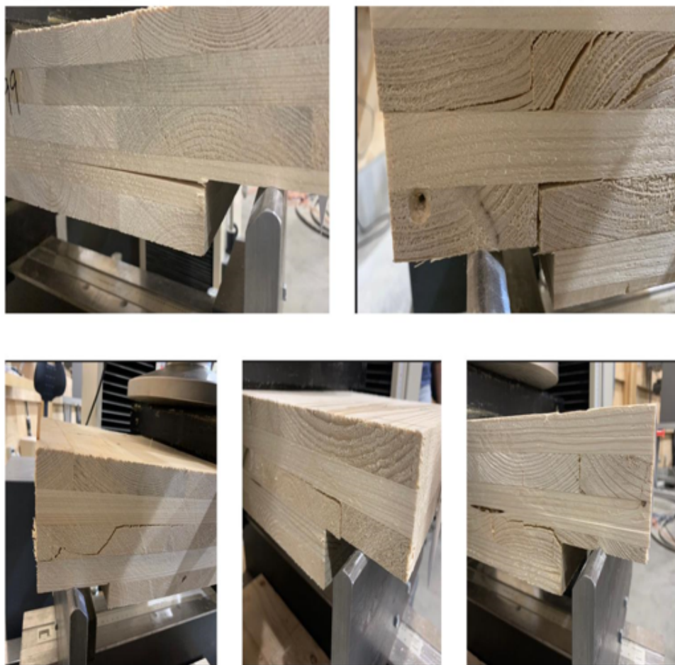
Figure 4: Different types of Shear Failures in 100mm series
